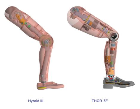
The THOR-5F femur has been designed with an axially compliant bushing which has been tuned to create a biofidelic response along the axis of the femur during a knee impact. The compliant section is constrained on a square shaft that slides linearly within a bushing.
