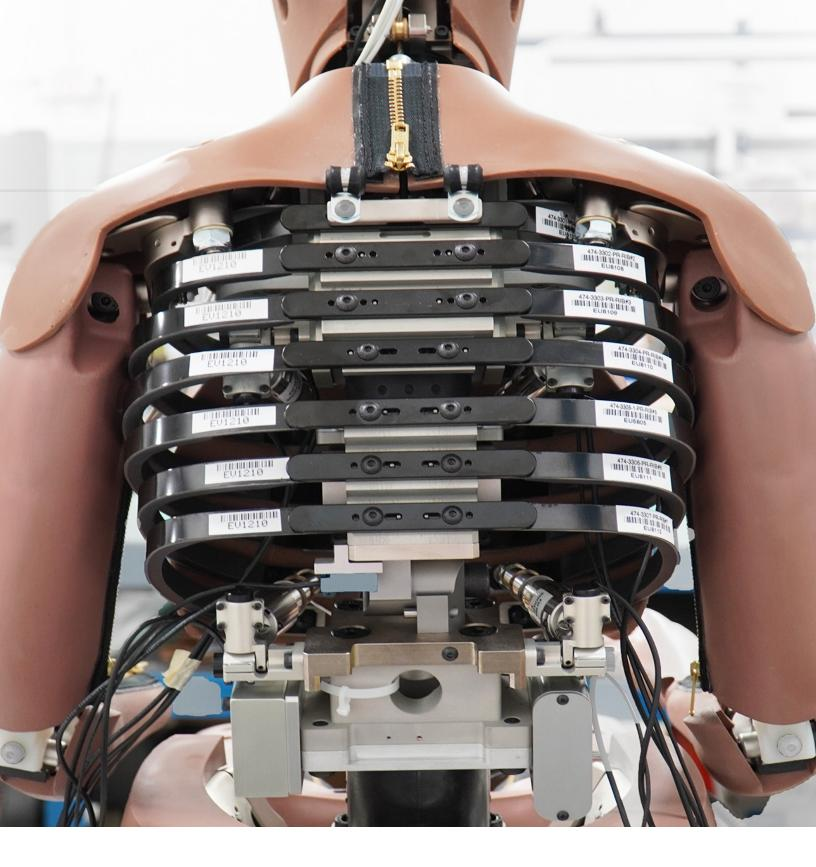
The THOR-5F is the first frontal Anthropomorphic Test Device (ATD) that is instrumented with sensors to measure impacts where women are most vulnerable to injury. The additional sensors enable a much more accurate understanding of injury risk and prevention.
