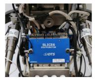
SLICE6 is the newest generation of in-dummy DAS for THOR. The ultra-small DAS reduces in-dummy cabling and connectors by up to 75%.
