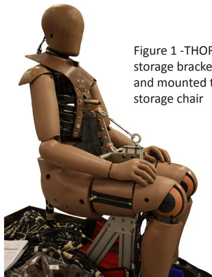
Figure 1 -THOR-M with storage bracket installed and mounted to the storage chair
